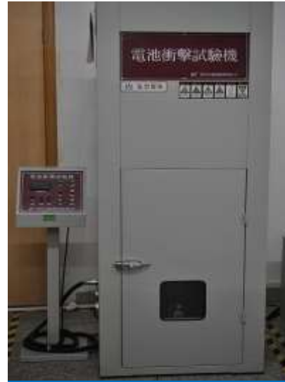
Impact testing machine
